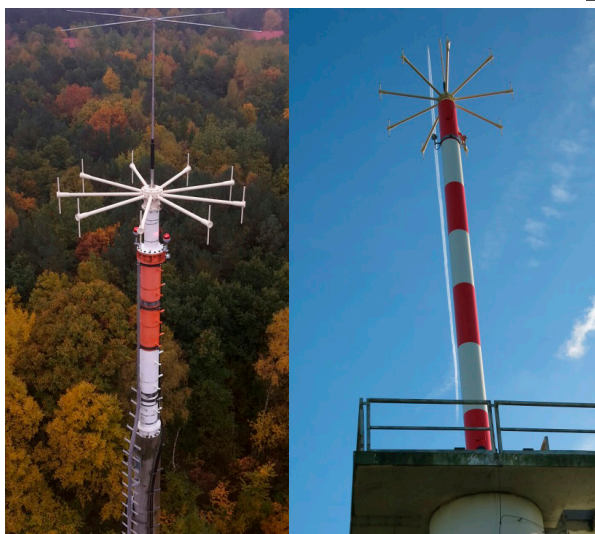
➤ The RDF antennas in Fassberg, Germany (L) and Beauvechain, Belgium (R) Photo: EUROCONTROL
